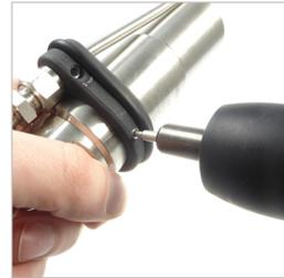
**Tightening torque 1 Nm**
