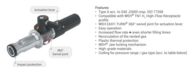
The WEH<sup>®</sup> TK16 H<sub>2</sub> High-Flow Fueling nozzle enables an even faster filling of buses and trucks with hydrogen. Due to the increased flow rate, the already short filling times have been shortened even further. The integrated swivel joint is located directly on the actuation lever, making it easy to rotate the fueling nozzle to the optimum connection position. The actuating lever can be switched with little effort when connecting and disconnecting.
