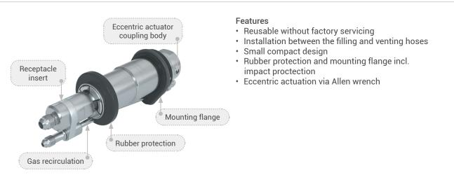
With the WEH<sup>®</sup> TSA2  $H_2$  Breakaway coupling, an inline breakaway coupling is also available for car refueling stations which is installed between the filling and venting hoses.
