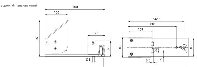
Mounting possibility for optionally available magnetic field sensor
