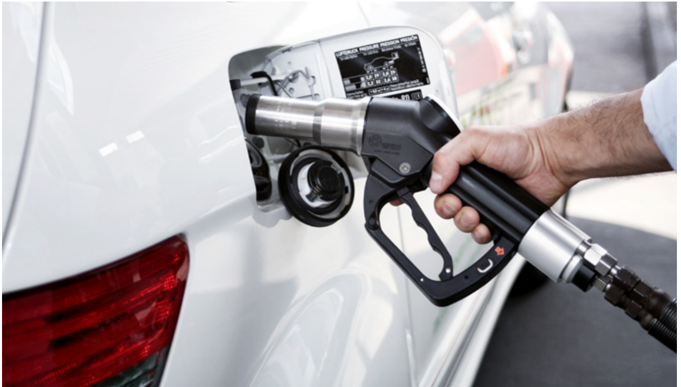
Car refueling with TK17 CNG
