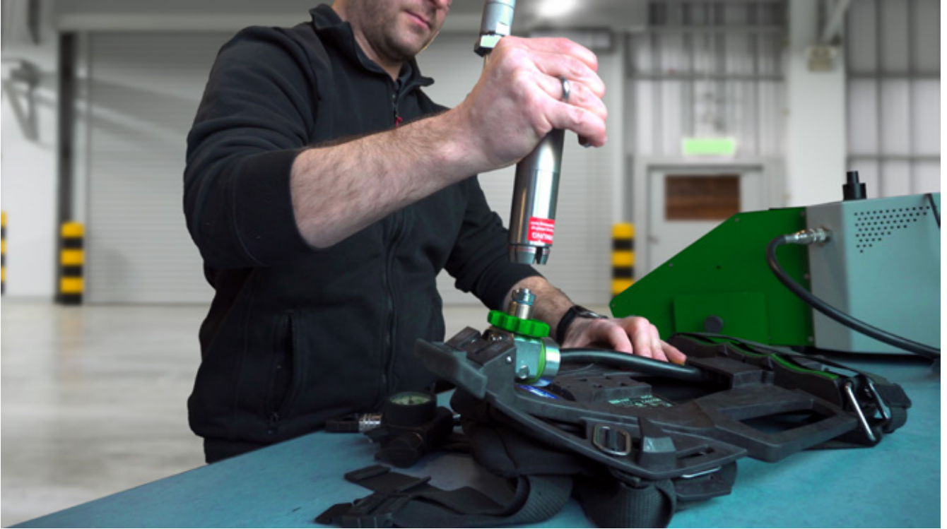
Testing respiratory protective equipment with WEH® connector TW156.
